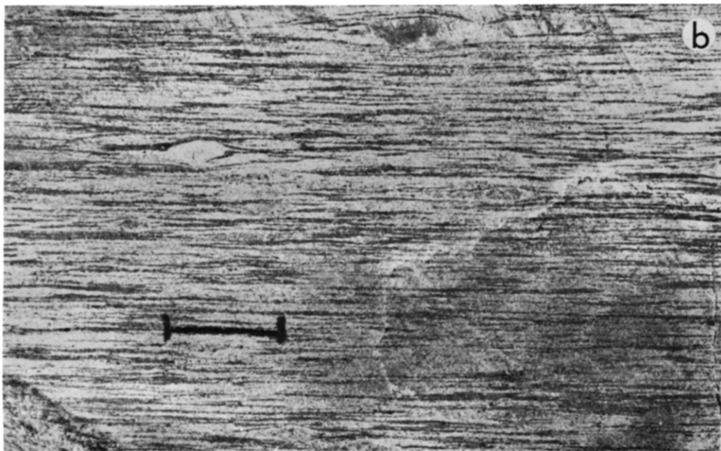
Fig. 7. Highly deformed quartzofeldspathic augen gneiss collected from the Piseco Dome. (a) View of foliation surface showing pronounced ribbons of quartz (dark) and K-feldspar (white). Scale bar is 2 cm. (b) Surface cut perpendicular to lineation and foliation. K-feldspar augen are almost all reduced to tails which appear as white layers and lenses. Dark layers of quartz indicate the large amount of elongation that has taken place. Scale bar is 2 cm long.
