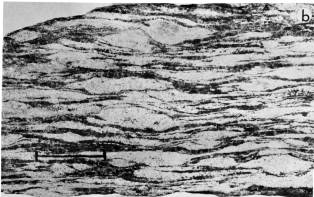
Fig. 6. Moderately deformed quartzofeldspathic augen gneiss collected from the Piseco Dome. (a) View of foliation surface showing good lineation and the development of ribbons of quartz (dark) and K-feldspar (white). Scale bar is 2 cm. (b) Surface cut perpendicular to lineation and foliation. K-feldspar augen have developed extensive tails with a consistent sense of asymmetry to foliation. Quartz aggregates (dark) have undergone considerable elongation. Scale bar is 2 cm long.
